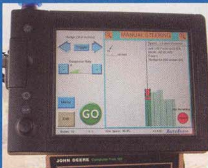
A new feature of the 2005 system, this touchscreen incorporates many of the electronics that were in the cab box.
