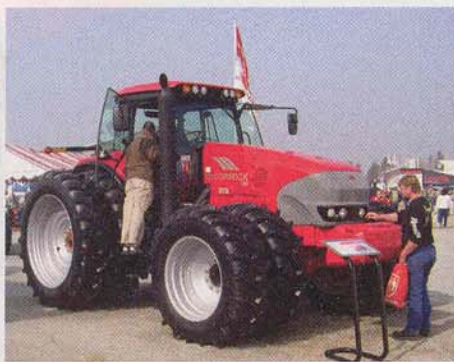
McCormick introduced its largest tractor yet, the ZTX with a 280-hp engine and an 18-speed powershift transmission.
