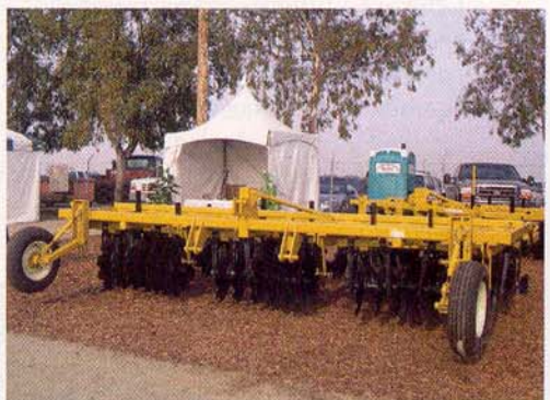
A bed reworking machine for minimum tillage in vegetable production was featured at the Hahn Tractor Company stand.
