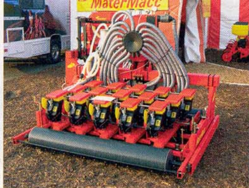
This high-density precision seeder from MaterMacc is used for planting on 80-inch beds.
