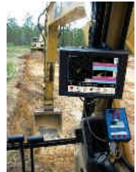
The Logic7D Excavate system as seen from the cabin
