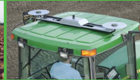
Multi-Antenna Roof Module
